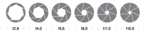
larger opening means sensor exposed to more light shallow depth of field smaller opening means sensor exposed to less light deep depth of field
